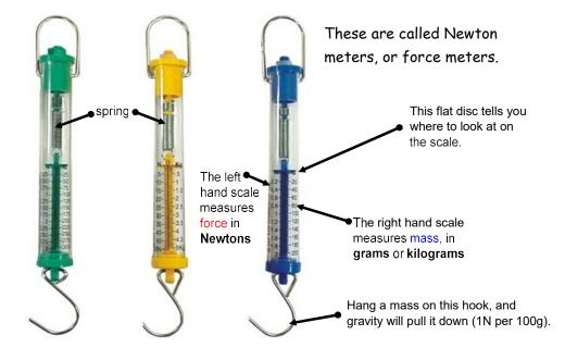
Different Newton meters have different ranges of measurements. Match up the maximum **mass** readings (g/kg) with the equivalent **force** readings (Newtons). Remember: gravity pulls on a mass of 100g with a force of 1N.
