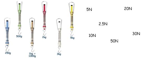
Unfortunately, because the maximum values are different for each Newton meter, each one has a different set of numbers so we need to work out how to read the scale before we use them.
