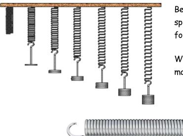
Because a pull force will stretch a spring, we can use it to measure the force of gravity on an object.
