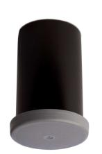
When the fizzing tablet was trapped inside the tub, the carbon dioxide gas had nowhere to escape. This meant that the  $CO_2$  particles filled the space more and more tightly, bouncing around the container and into each other with ever more force. This created **pressure** inside the tub, causing the lid and base to bulge out.
