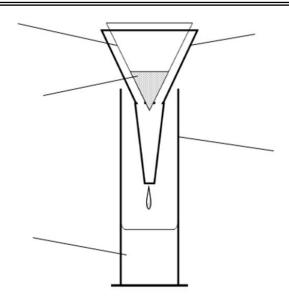
Using filtration to separate solids and liquids
